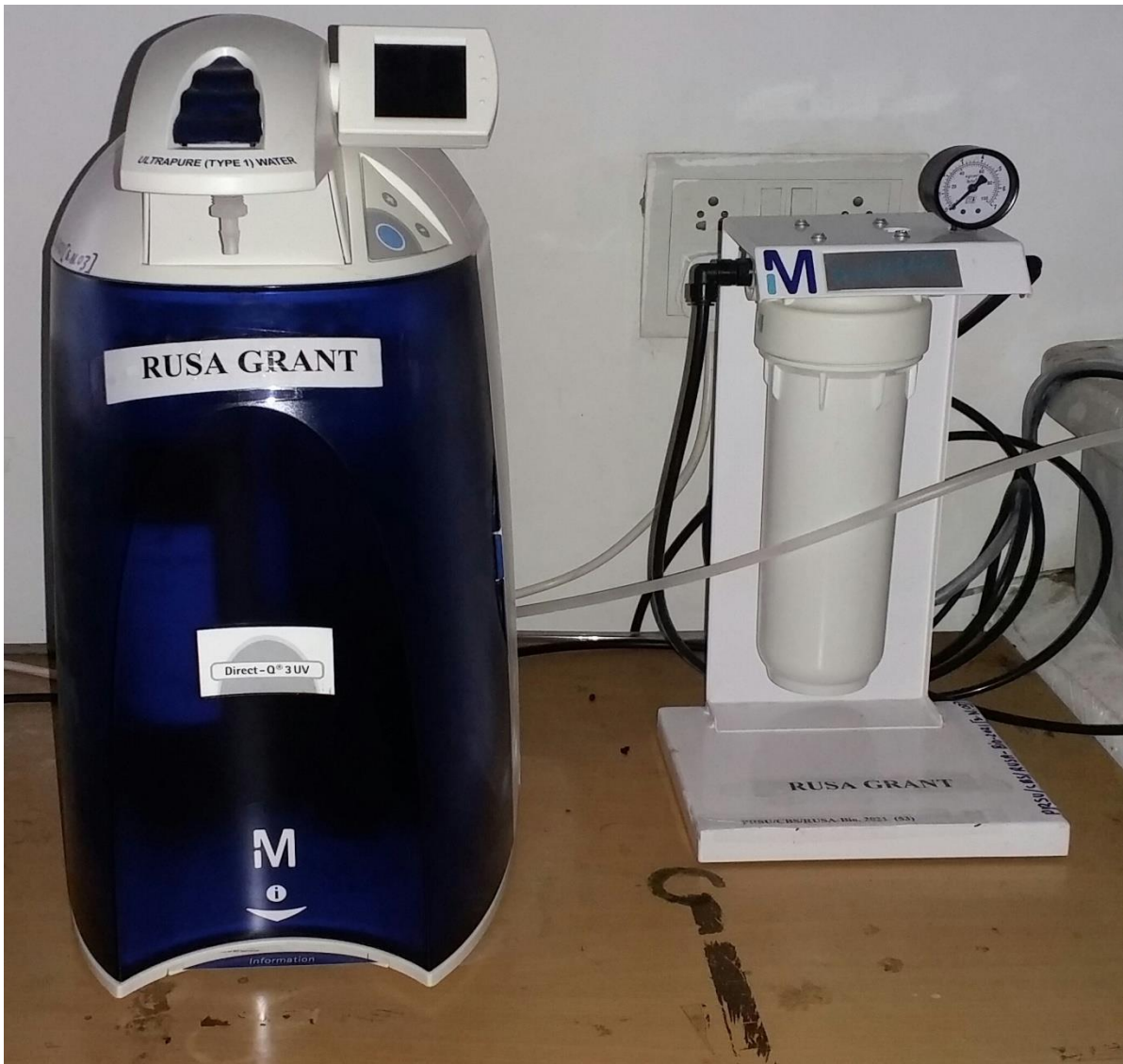
Fig.01. Water Purification System
