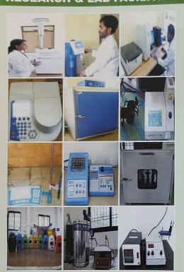
Department has many sophisticated instruments such as Ion Chromatography, Ion Selective Electrode, UV Visible Spectrophotometer, CO2 Meter, Bacterial Incubator, High volume Air sampler, Sound meter, Flame Photometer, Meteorological Sensor, Deep Freezer, Water Purification, Bomb Calorimeter, Water Distillation etc.
